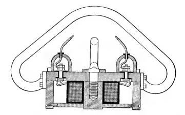
FIG. 50. Cross-section of a lifting magnet such as is used for lifting heavy safes, etc. (El. Controller & Supply Co.)
